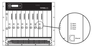
The system is ready for configuration once the Power and the Active LED are green and the initial configuration menu appears on the LCD.
